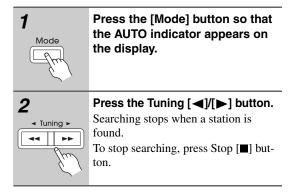
When tuned into a station, the ▶ • ◀ indicator appears. When tuned into a stereo FM station, the FM ST indicator appears on the display, as shown.
